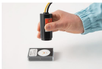
● Validate probe functionality with Probe Checker
